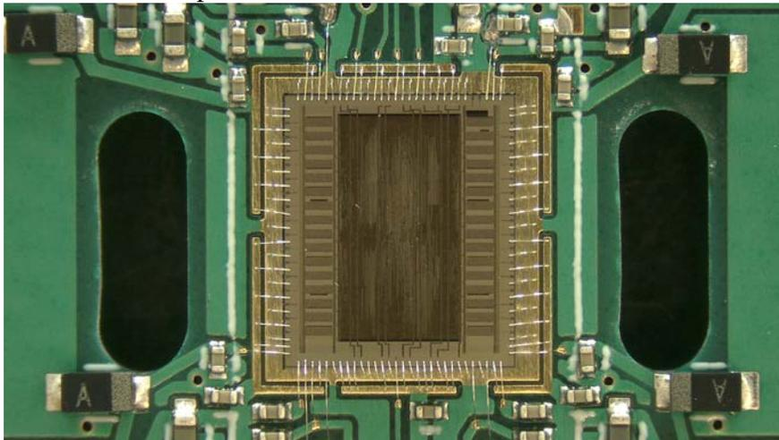
*Figure 6: 32-channel custom-designed IC at LBNL for reading out pixels of LArTPC.*
