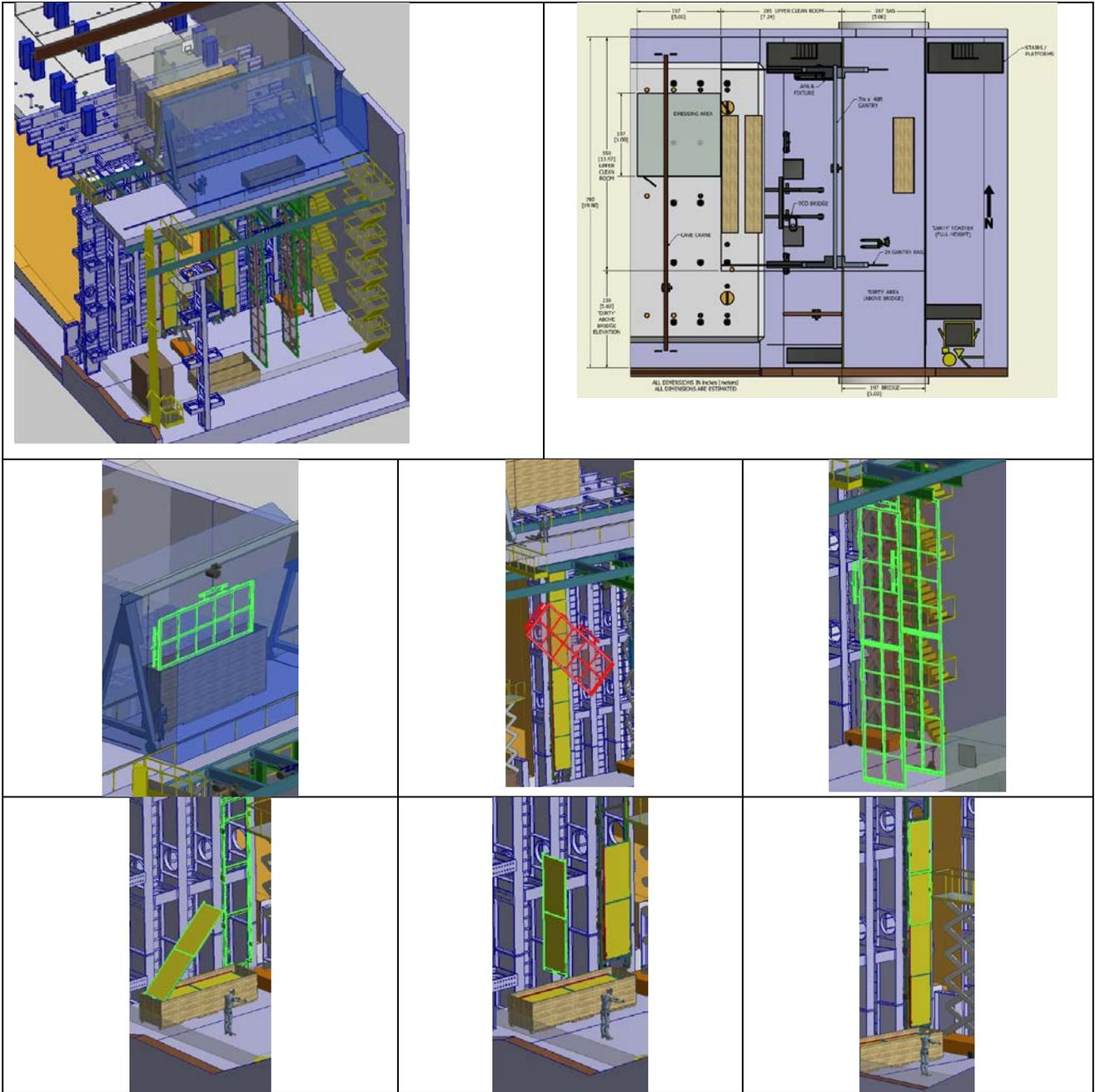
*Figure 8: Installation concept if the rock pillar is removed and the space reduced to 12m.*
