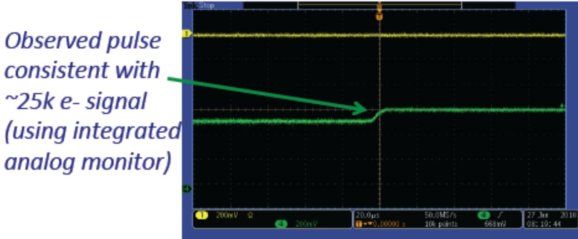
Figure 7: Detected 25k-electron signal with LArPix.
