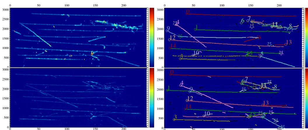
**Figure 7:** (left) Raw hits of an event obtained with LArASIC, (right) Reconstructed 19 tracks of the event.
