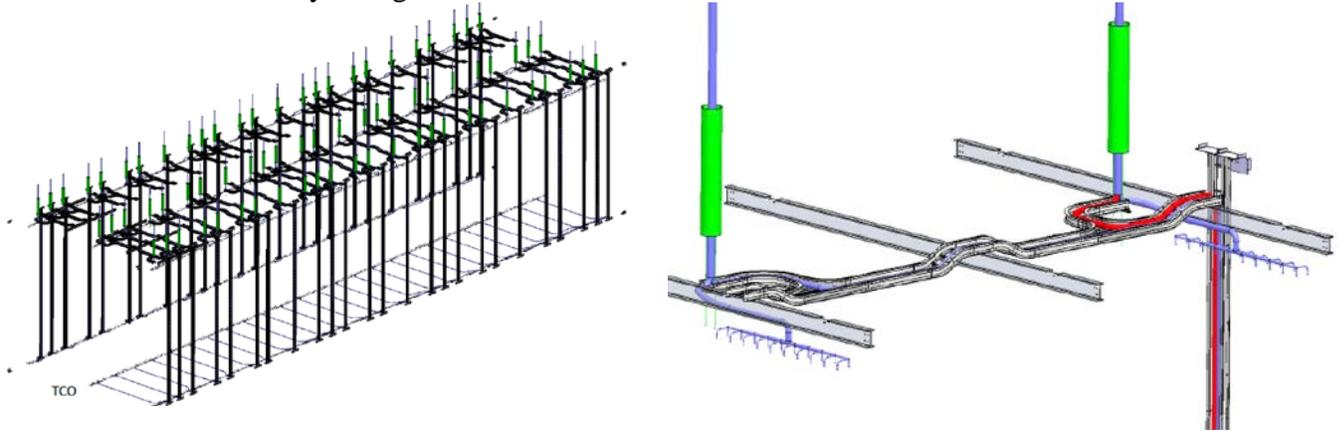
*Figure 7: Left: Full 3D model of the cable routing with cable trays along the walls of the cryostat. Right: Detail view of one tray at the top of the detector (for 2 APAs). The top trays are supported from the DSS I-Beams and the cryostat wall trays are supported from M10 bolts in the edges of the cryostat.*
