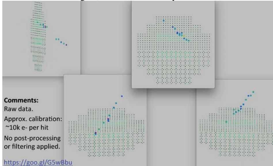
**Figure 8:** Cosmic-ray muon tracks observed with the LBNL low-power LArPix ASIC.
