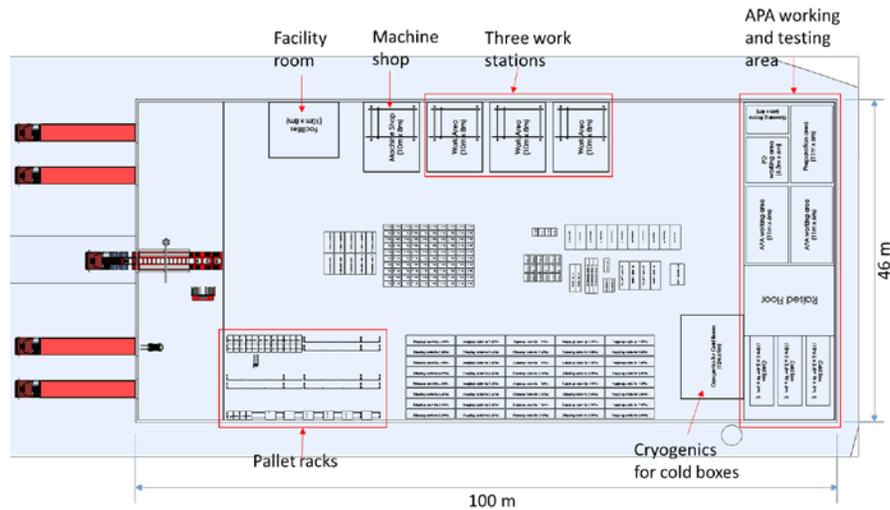
*Figure 6: Conceptual ITF layout with functional regions indicated. This gives an indication of the space needs. This layout considers space available on a potential lot near SDSM&T.*
