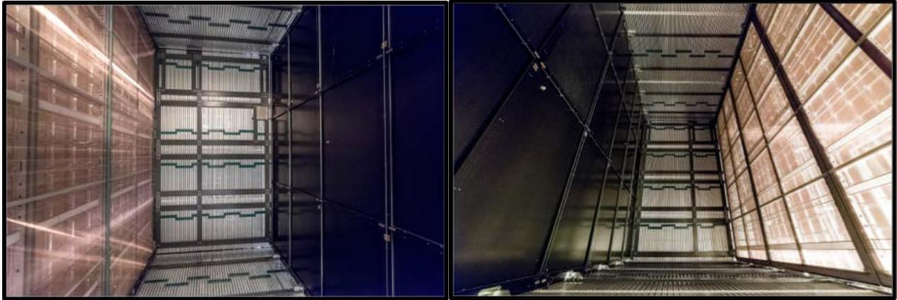
*Figure 4: ProtoDUNE-SP field cages completed*
