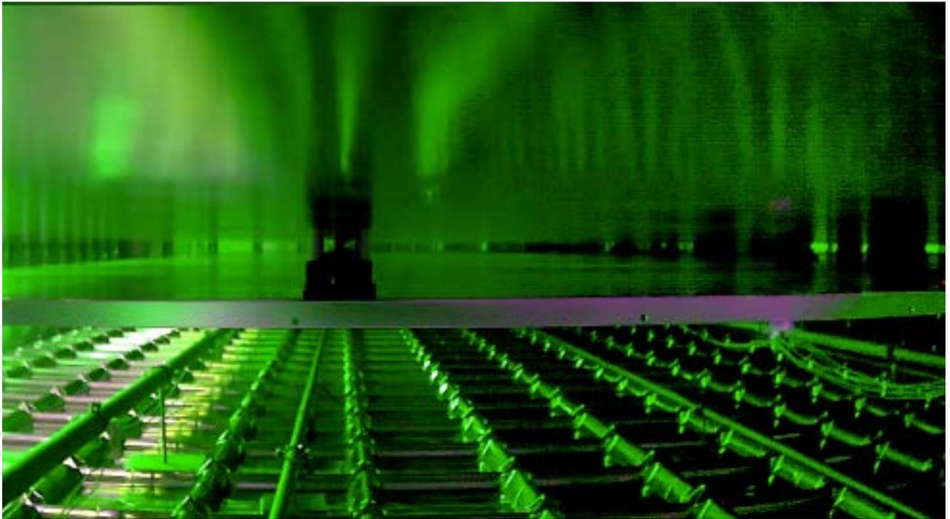
**ProtoDUNE-SP liquid argon level above the lower ground plane**
