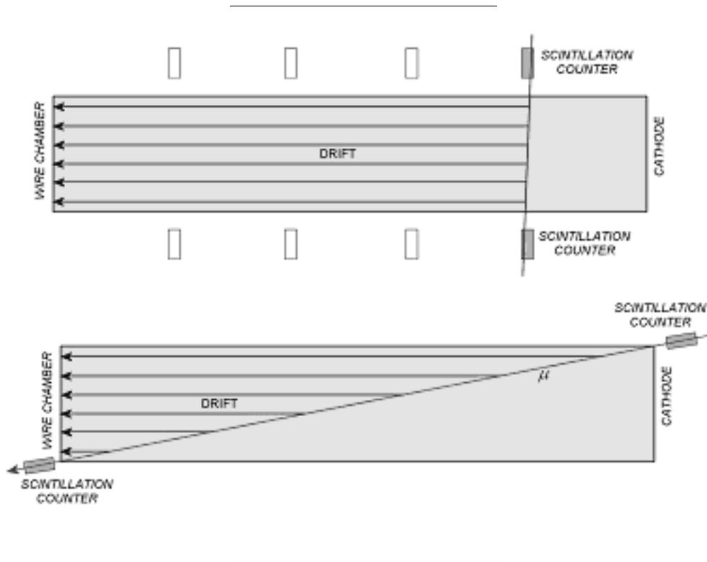
Figure 5: Collecting event with vertical cosmic ray trigger (top) and Collecting event with muon beam inclined with respect to the drift direction (bottom).
