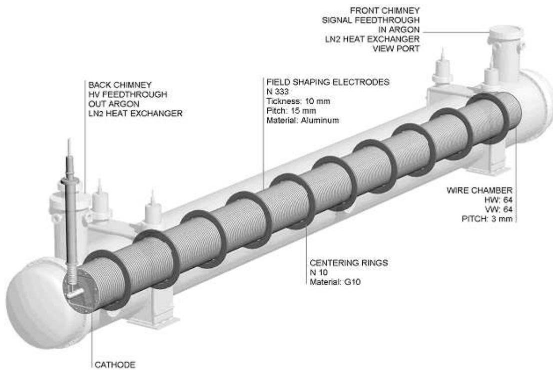
Figure 6: The 5-m drift time projection chamber.
