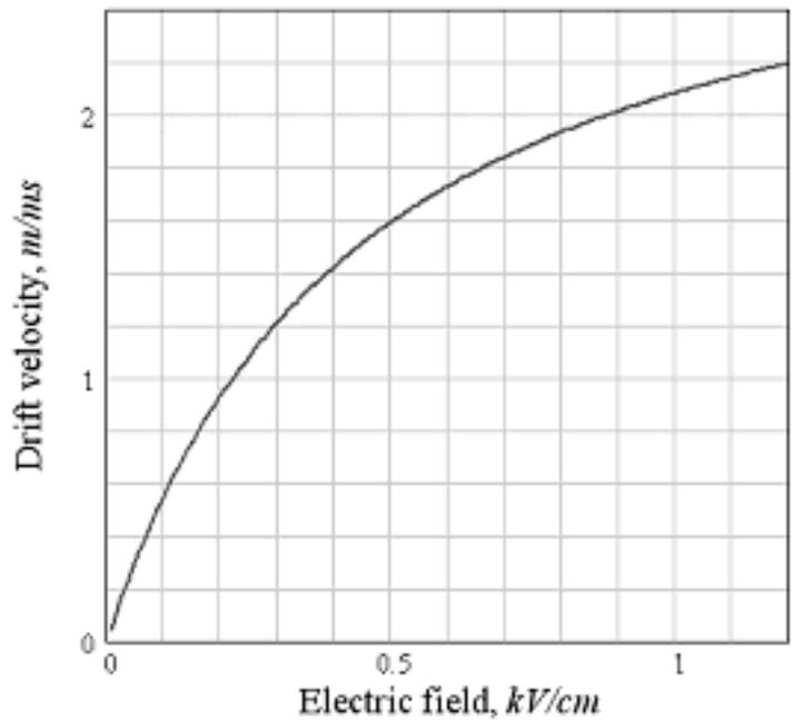
Figure 4: Drift velocity versus electric field in liquid Argon.
