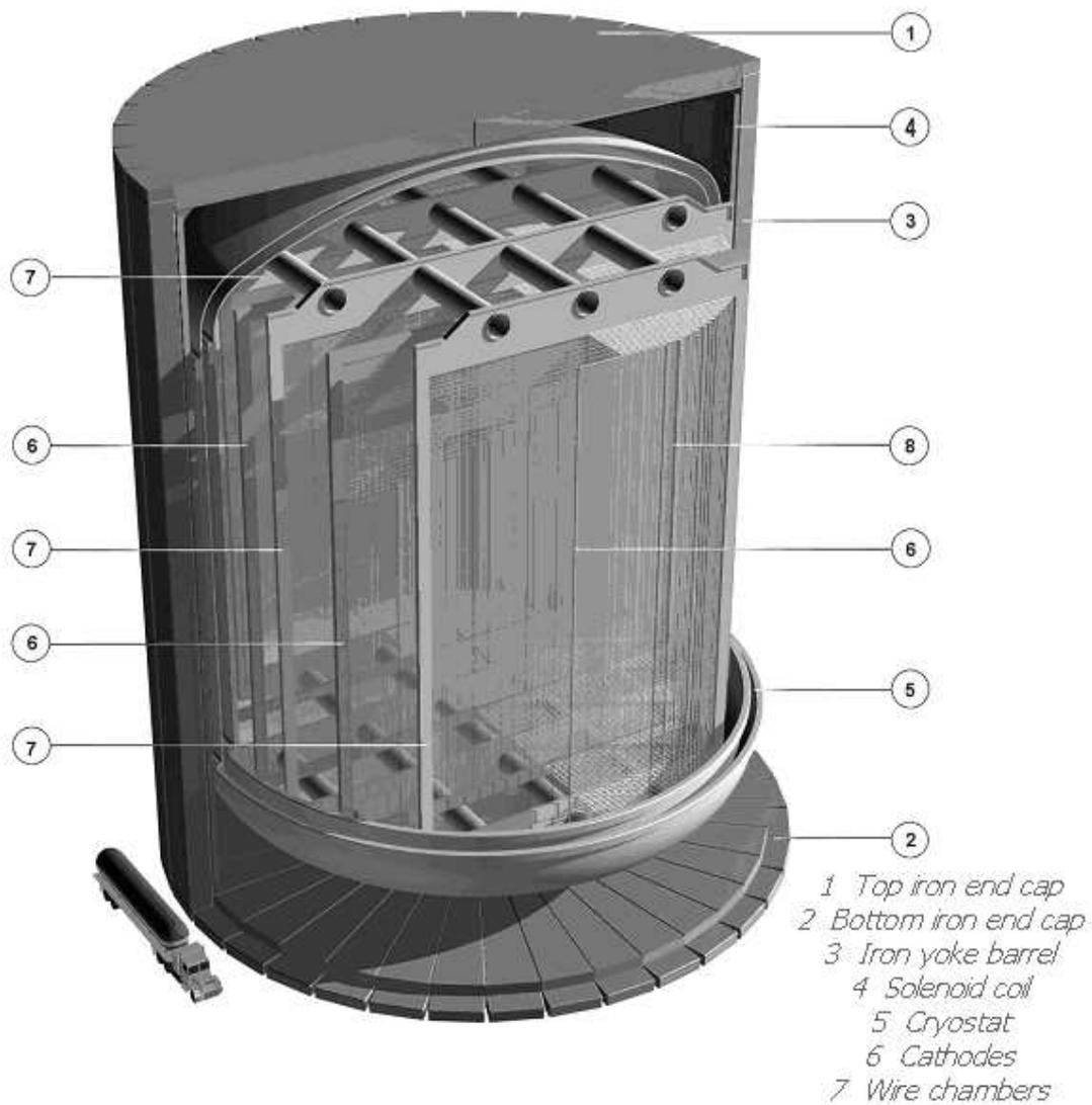
Figure 3: Cutaway view of the LANNDD detector.
